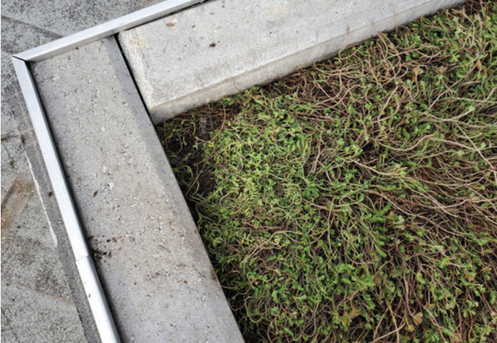
FIGURE 7 - Sedum plants did not suffer much damage after the wind flow test.
