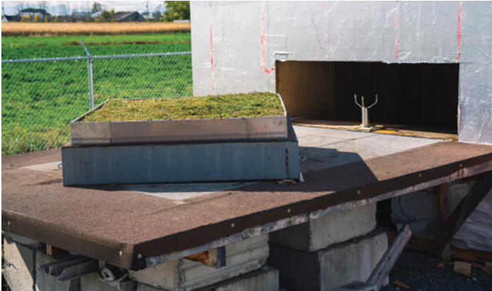
FIGURE 5 - A vegetated mat system is ready for wind flow testing.
