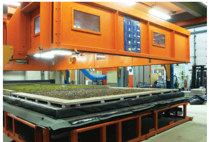
FIGURE 4 - A vegetated mat system is ready for wind uplift testing.
