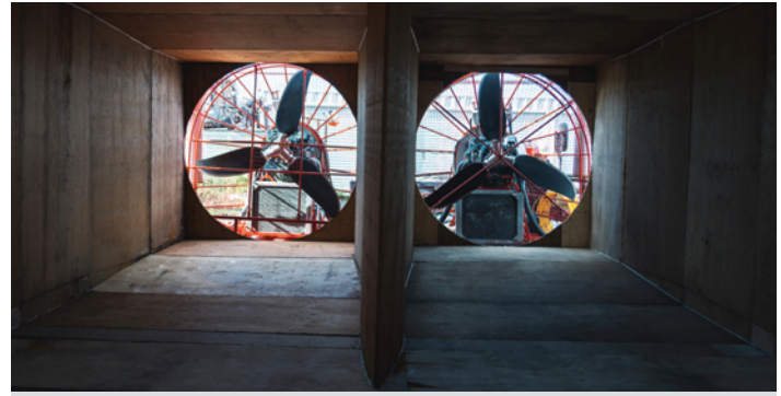
FIGURE 6 - The airflow machine generated wind using twin fans.
