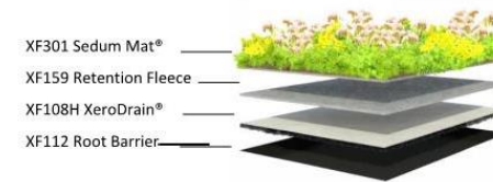
Figure 1 Principal components of the XF301 system
